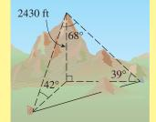
**6. Determining a Distance** A surveyor has determined that a mountain is 2430 ft high. From the top of the mountain he measures the angles of depression to two landmarks at the base of the mountain, and finds them to be 42° and 39°. (Observe that these are the same as the angles of elevation from the landmarks as shown in the figure at the left.) The angle between the lines of sight to the landmarks is 68°. Calculate the distance between the two landmarks.
