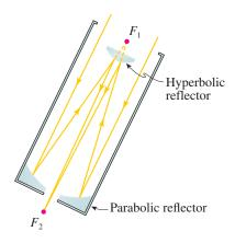
**Figure 8**Cassegrain-type telescope
