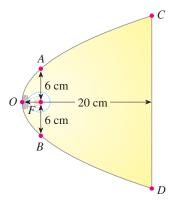
**50. Satellite Dish** A reflector for a satellite dish is parabolic in cross section, with the receiver at the focus *F*. The reflector is 1 ft deep and 20 ft wide from rim to rim (see the figure). How far is the receiver from the vertex of the parabolic reflector?
