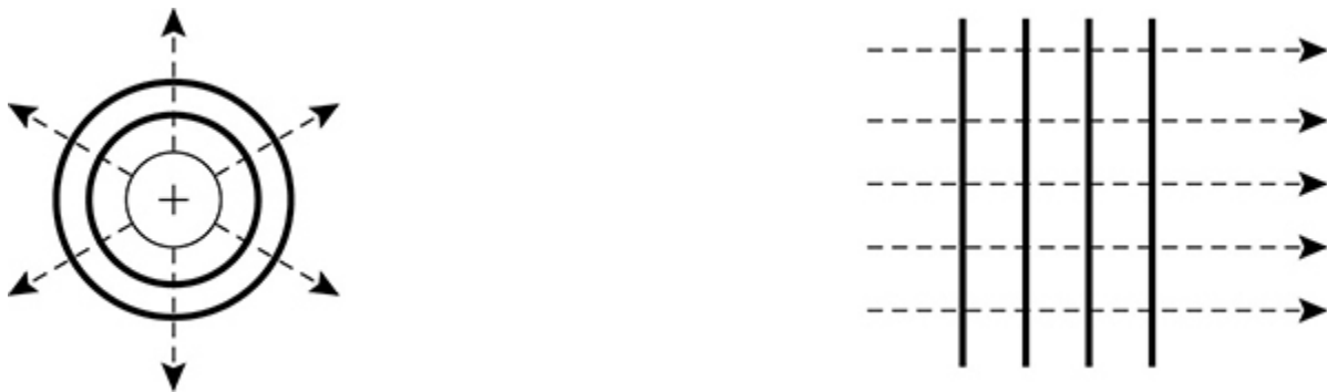
Figure 17.2 Two examples of equipotential lines (in bold) and electric field lines (dotted).
