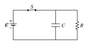
14. Identical resistors and identical uncharged capacitors are connected to identical ideal batteries of a fixed emf shown in the circuits given. Each circuit has a switch S in the open position. In which circuit will the capacitors charge in the least amount of time when switch S is closed?
