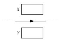
If the current in the wire is constant, and the wire is moved towards loop X, what is the direction of the induced current, if any, in each of the loops?
