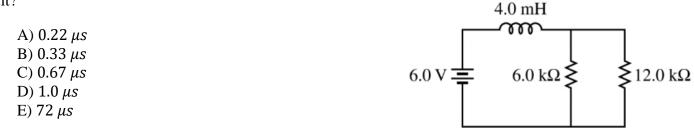
13. For the circuit shown, what is the rate of change of the current in the inductor when the current in the battery is 0.50 A?
