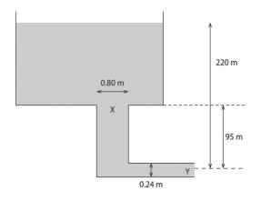
4. In the diagram below shown the exit at Y is opened so that Y is exposed to atmospheric pressure.  $(\rho_{WATER} = 1000 \frac{kg}{m^3})$
